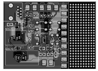
Figure 50. AD5171 Evaluation Board
