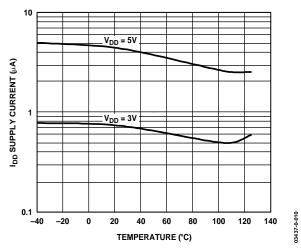
Figure 11. Supply Current vs. Temperature
