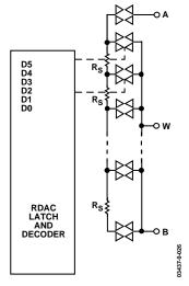
Figure 31. AD5171 Equivalent RDAC Circuit
