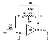
Figure 41. Typical Noninverting Gain Amplifier
