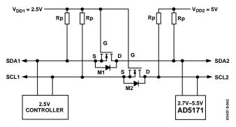
Figure 43. Level Shifting for Different Voltage Operation
