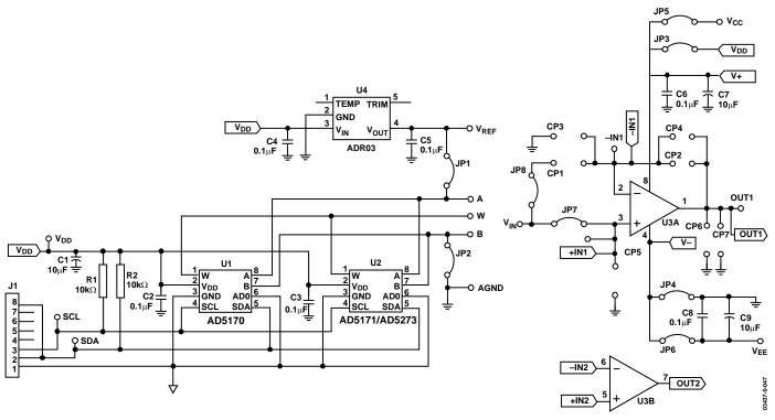
Figure 48. AD5171 Evaluation Board Schematic
