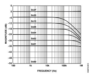
Figure 16. Gain vs. Frequency vs. Code,  $R_{AB} = 50 \Omega$
