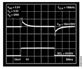
Figure 19. Digital Feedthrough vs. Time
