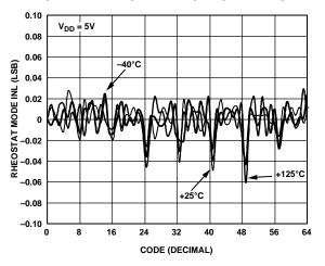
Figure 5. R-INL vs. Code vs. Temperature
