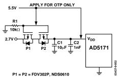
Figure 27. Isolating the 5.5 V OTP Supply from the 2.7 V Normal Operating Supply. The  $V_{\rm DD}$  or supply must be removed once OTP is complete.
