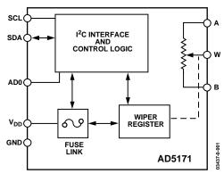
Figure 1. Functional Block Diagram
