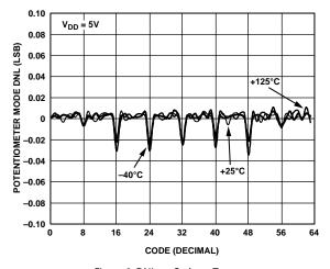
Figure 8. DNL vs. Code vs. Temperature
