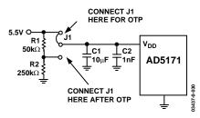
Figure 25. Power Supply Requirement
