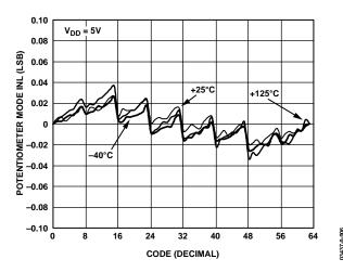
Figure 7. INL vs. Code vs. Temperature
