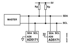
Figure 39. Two AD5171 Devices on One Bus
