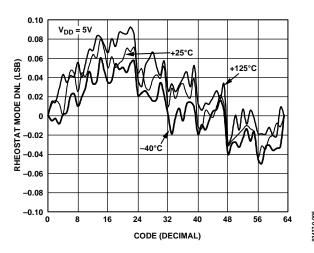
Figure 6. R-DNL vs. Code vs. Temperature
