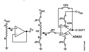
Figure 49. Programmable Voltage Reference
