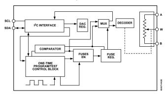
Figure 24. Detailed Functional Block Diagram
