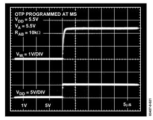
Figure 22. Power-Up Settling Time, after Fuses Blown
