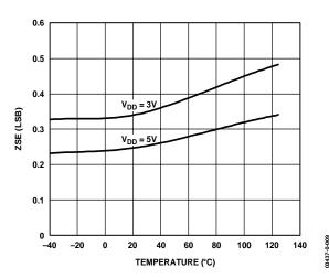
Figure 10. Zero-Scale Error
