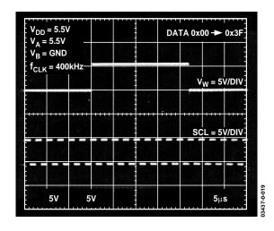
Figure 20. Settling Time
