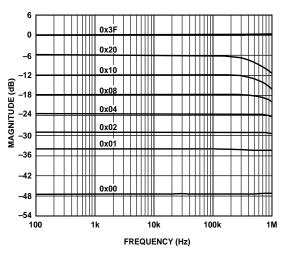
Figure 15. Gain vs. Frequency vs. Code,  $R_{AB} = 10 \text{ k}\Omega$
