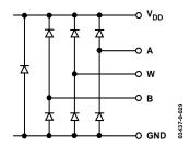
Figure 29. Maximum Terminal Voltages Set by VDD
