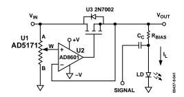
Figure 42. Programmable Booster Voltage Source
