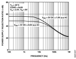
Figure 18. PSRR vs. Frequency
